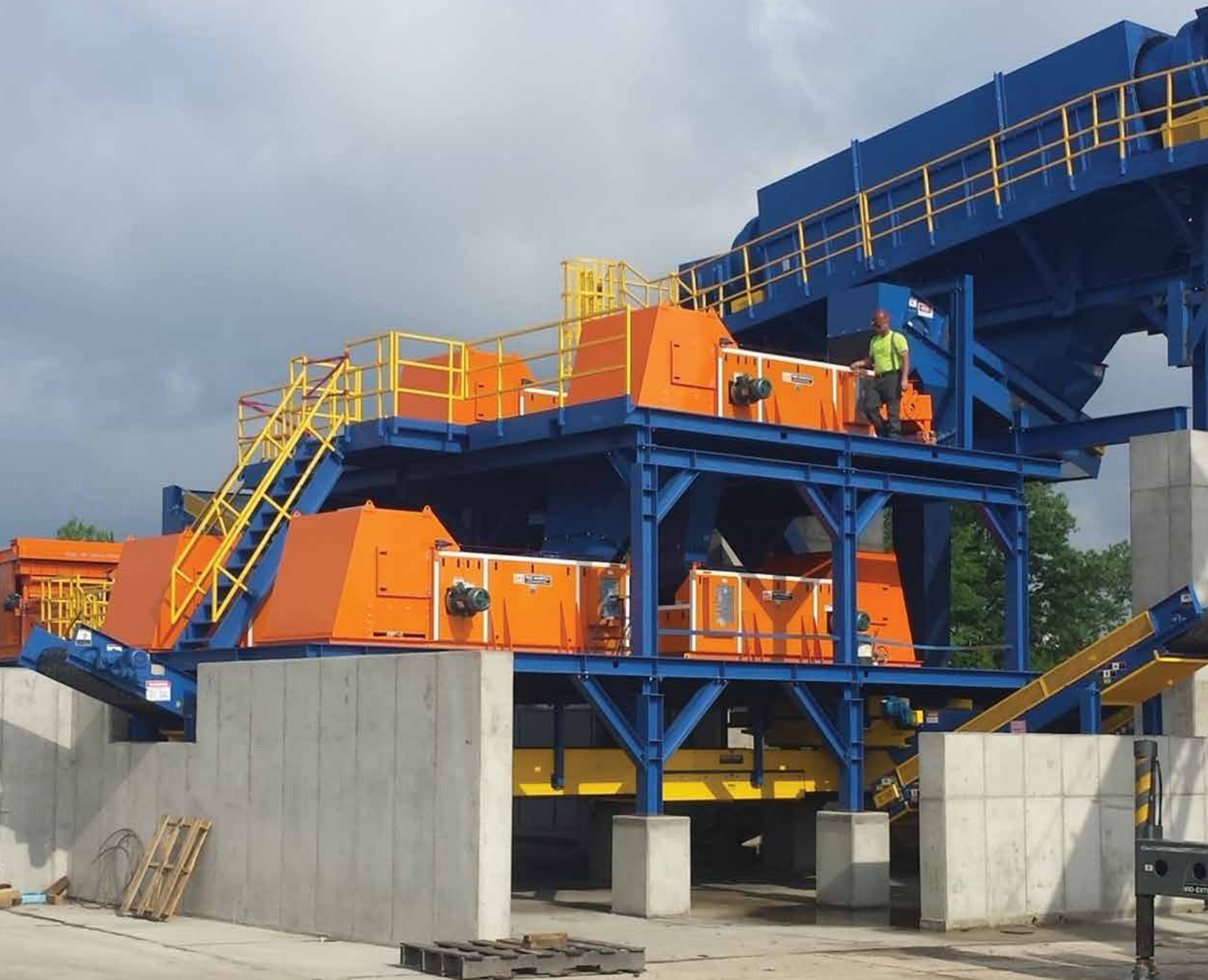
A scrap yard in Ohio employs a number of Eriez' RevX-E Eddys to ensure maximum recovery in their facility
