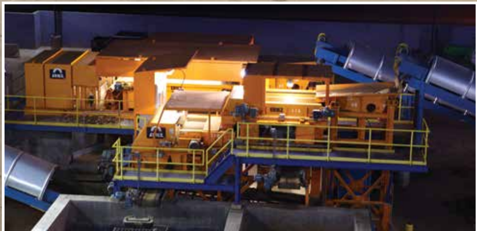
An auto scrap recycler in Arizona sorts nonferrous and fines using Eriez' RevX-E Eddys
