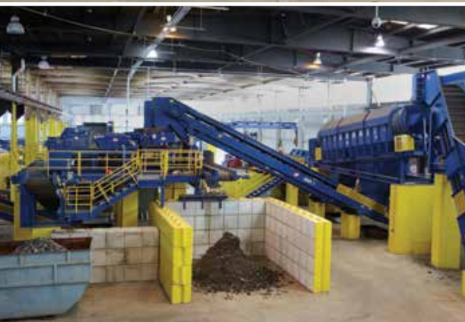
Side-by-Side Eddy Current Separators recover Zorba from ASR screened by an upstream trommel screen.
