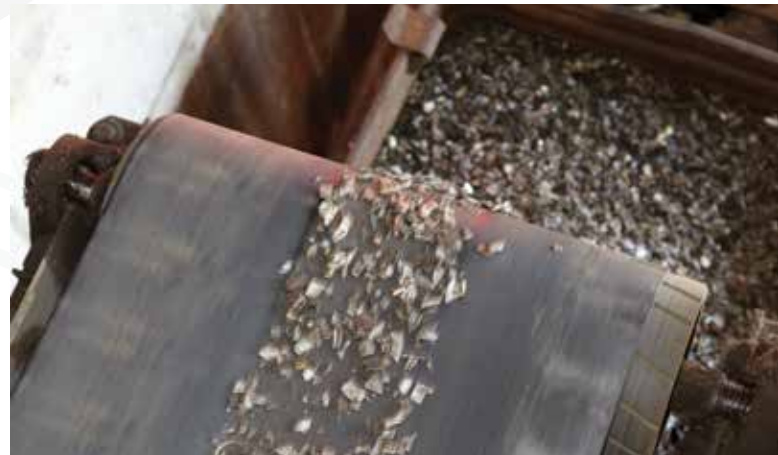
Fine non-ferrous metals are recovered to produce a high value Zorba product at Auto Shredder Residue (ASR) plants.
