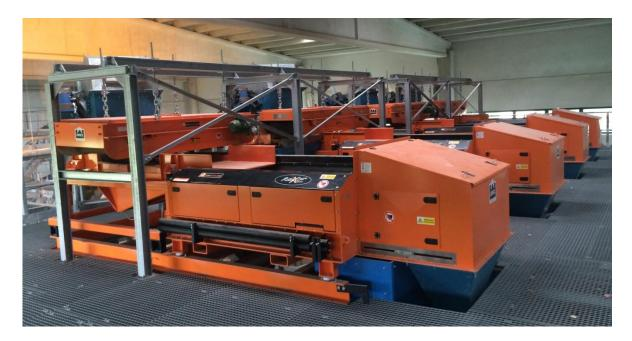
For complete metal recovery, Eriez manufacture a range of modular systems to separate ferrous and non-ferrous metals, designed to incorporate additional separators including overband magnets and magnetic drums, into stand-alone systems.
