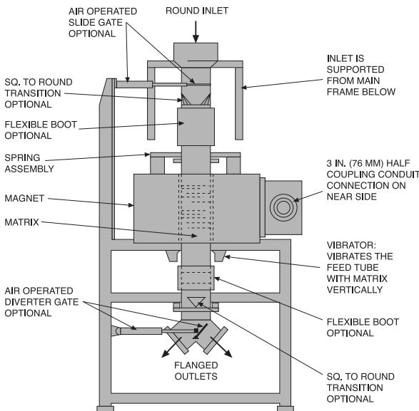
**Figure 1:** Dry Vibrating Magnetic Filters are designed specifically for dry applications - the treatment of powders. Its purpose is to remove fine ferrous contaminants from dry powder.
