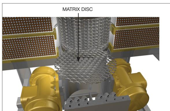
**Figures 2 and 3:** The DVMF consists of a thick steel box with a canister in the bore. Aluminum or copper coils are positioned around the canister. Direct current power energizes the coil and allows the matrix to collect magnetic particles.
